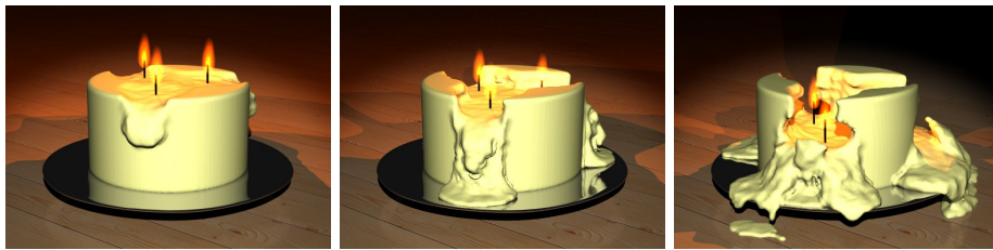
Figure 7.8: A burning candle simulation showing melting and re-solidifying of wax. The particle’s temperature is used to fade between the elastic and liquid regime.
