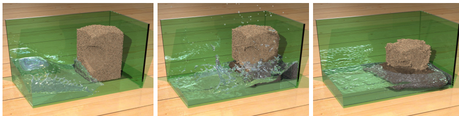
Figure 6.12: A moist sand column stands rigidly until a column of water is released. The water percolates through the sand and erodes pieces of the structure.
