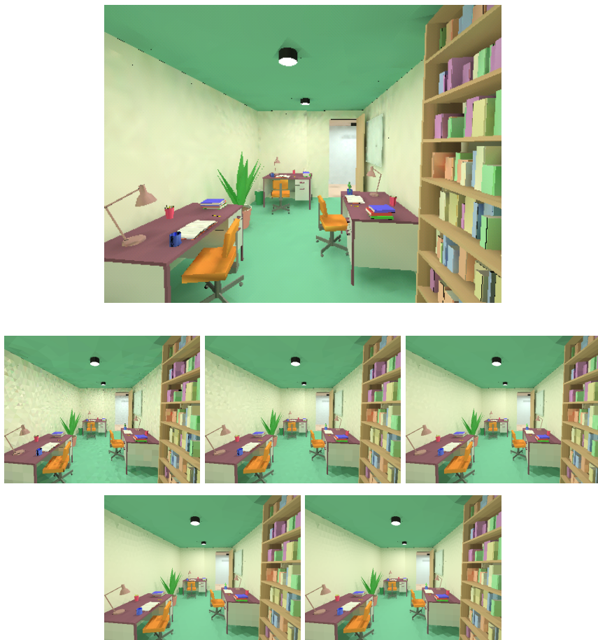
Figure 6.1: Stochastic relaxation methods can yield useful images much faster than their deterministic counterparts. The shown environment consists of slightly more than 30,000 patches. The top image was obtained with incremental Jacobi iterations in less than 2 minutes using about 10^6 rays. Even if only 1 ray were used for each form factor, 9 \cdot 10^8 rays would be required with a deterministic method. Noisy artifacts are still visible, but are progressively reduced. After about 30 minutes, they are not visible anymore. The bottom images illustrate progressive variance reduction using regular Jacobi iterations after a first sequence of incremental iterations. The images are shown without Gouraud shading, so noisy artifacts are more visible. The images shown are obtained after 1, 4, 16, 64 and 252 (right-to-left, top-to-bottom) iterations of less than 2 minutes each. The model shown is an edited part of the Soda Hall VRML model made available at the University of California at Berkeley, U.S.A.
